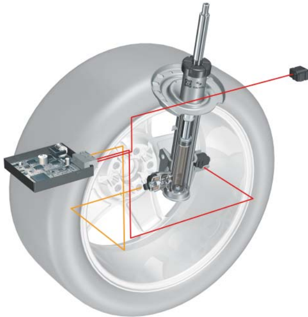
Figure 18.11 CDC: Continuous damping control (reproduced with permissions of ZF Friedrichshafen AG)
