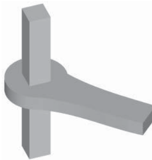
Figure 20.4 Translational joint or prismatic joint
