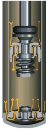
Figure 18.6 Twin-tube shock absorber: details of flow for rebound (reproduced with permissions of ZF Friedrichshafen AG)
